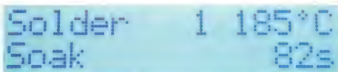
Figure 9. Status display of a solder cycle in process.
